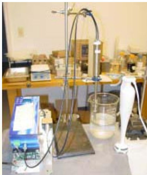
Figure 1: Test apparatus. The homogenizer is shown outside the test solution for clarity. During testing, the homogenizer was clamped in place and not removed from the solution.
