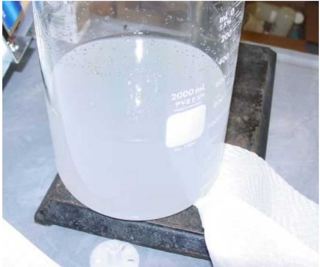
Figure 4: 200 PPM of EPA #2 oil homogenized for 1 minute.
