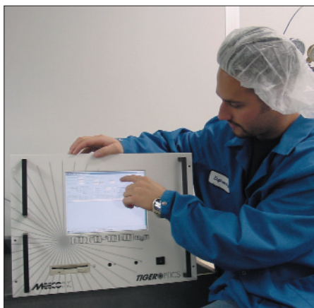
Tiger Optics’s CRDS system in action: the MTO-1000 can measure moisture levels of 100 ppt.
